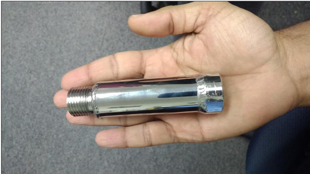
**Figure 3:** An NLP water “conditioner” that claimed to soften water without any treatment chemicals did not perform as advertised in a battery of laboratory tests conducted by our team.
